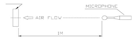
4. NOISE IS MEASURED AT RATED VOLTAGE IN FREE AIR IN A SEMI-ANECHOIC CHAMBER WITH A & D SOUND LEVEL METER WITH MICROPHONE AT A DISTANCE OF ONE METER FROM THE FAN INTAKE.
