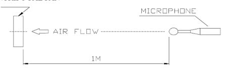
4. NOISE IS MEASURED AT RATED VOLTAGE IN FREE AIR IN A SEMI-ANECHOIC CHAMBER WITH A & D SOUND LEVEL METER WITH MICROPHONE AT A DISTANCE OF ONE METER FROM THE FAN INTAKE.
