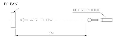
4. NOISE IS MEASURED AT RATED VOLTAGE IN FREE AIR IN A SEMI-ANECHOIC CHAMBER WITH A & D SOUND LEVEL METER WITH MICROPHONE AT A DISTANCE OF ONE METER FROM THE FAN INTAKE.
